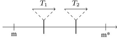
(a) Interacting preemptions by  $T_1$  and  $T_2$  between two subsequent accesses to  $m$ .
