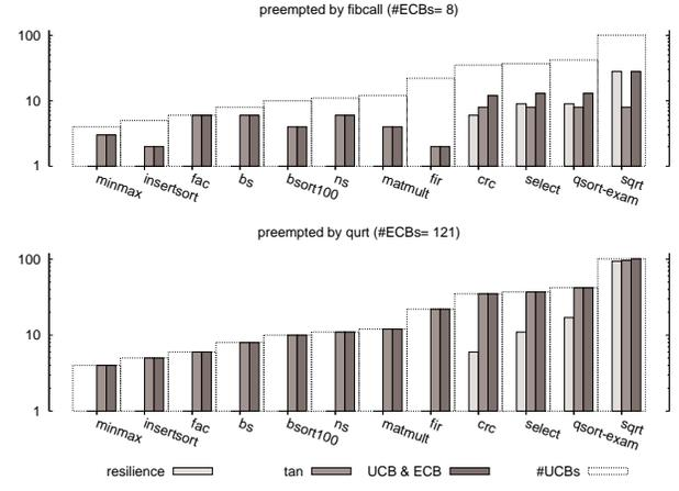
**Figure 6.** Number of additional misses due to preemption by *fibcall* and *qurt* when the CRPD is computed with Equations 10 (resilience), 7 (UCB & ECB), 8 (Tan) and 1 (#UCBs).
