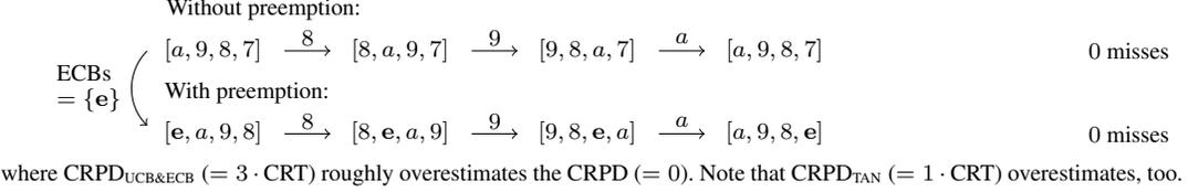
**Figure 1.** Evolution of the cache contents for LRU replacement. The first row shows the evolution of the cache contents for one iteration of the loop without preemption. The second row shows the evolution of the cache contents on the same sequence with preemption. The preempting task accesses block  $e$ . A \* as in  $a^*$  indicates a miss.
