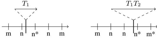
(c) Isolated preemptions by  $T_1$  and  $T_1T_2$ . The sum of the number of additional misses,  $1 + 2 = 3$ , bounds the number of additional misses in case of interacting preemptions, 3, by  $T_1$  and  $T_2$  as depicted in (b).
