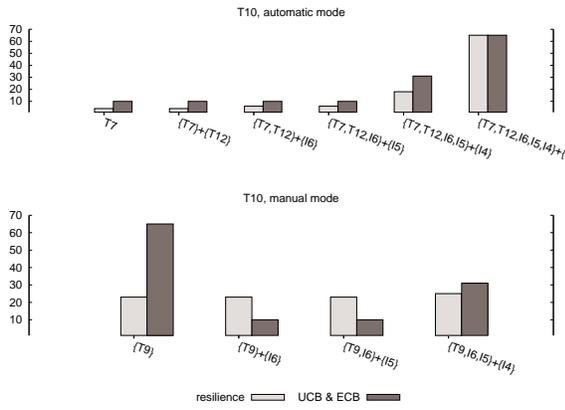
**Figure 7.** Bounds on the number of additional misses of task T10 due to a single preemption 1) by a set of tasks (resilience), e.g. {T9, I6, I5} and 2) by a single task (UCB&ECB), e.g. I5.
