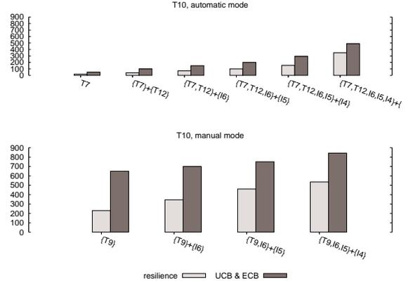
**Figure 8.** Bounds on the number of additional misses of task T10 due to preemptions by sets of tasks, derived by Resilience and UCB&ECB. These are weighted sums of the results for single preemptions which are shown in Figure 7.
