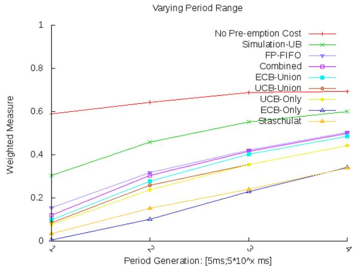
Fig. 28. Weighted schedulability measure; varying the range of task periods  $[5, 50]$  to  $[5, 5 \cdot 10^4]$  (constrained deadline)
