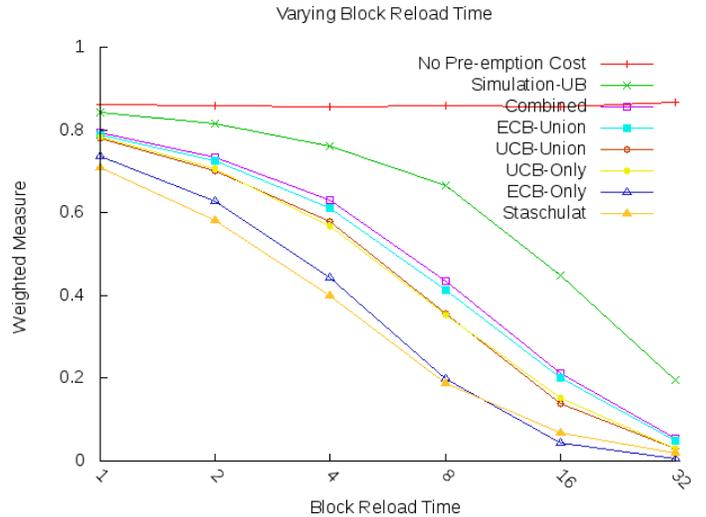
Fig. 11. Weighted schedulability measure; varying block reload time from  $2^0 = 1\mu s$  to  $2^4 = 32\mu s$
