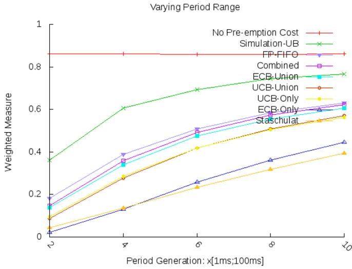
Fig. 21. Weighted schedulability measure; varying the scale of task periods  $w[1, 100]$  from  $w = 2$  to  $w = 10$  (with FP-FIFO)
