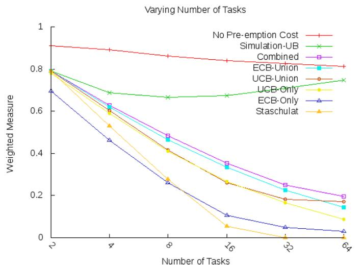
Fig. 9. Weighted schedulability measure; varying number of tasks from  $2 = 2^1$  to  $2^6 = 64$ .
