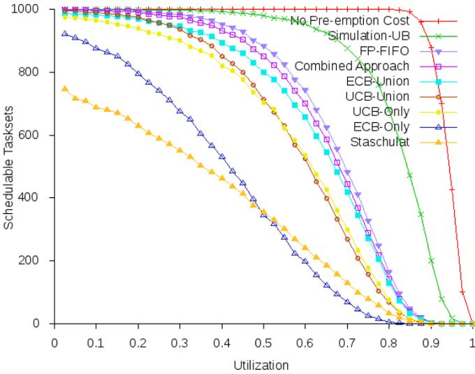
Fig. 14. Evaluation of base configuration. Number of tasksets deemed schedulable at the different total utilizations (with FP-FIFO).
