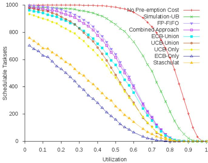
Fig. 22. Evaluation of base configuration. Number of tasksets deemed schedulable at the different total utilizations (constrained deadline).
