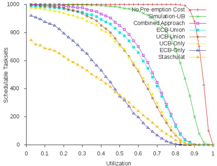
Fig. 6. Evaluation of base configuration. Number of tasksets deemed schedulable at the different total utilizations.
