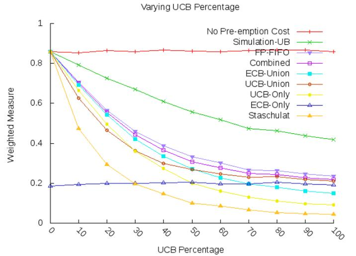
Fig. 16. Weighted schedulability measure; varying reuse factor from 0% to 100%, in steps of 10% (with FP-FIFO)
