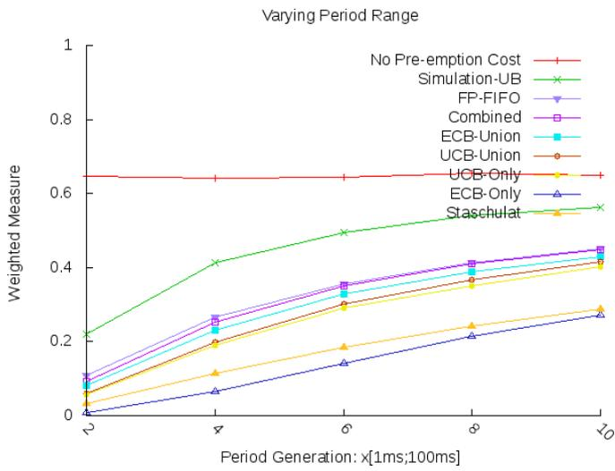
Fig. 29. Weighted schedulability measure; varying the scale of task periods  $w[1, 100]$  from  $w = 2$  to  $w = 10$  (constrained deadline)
