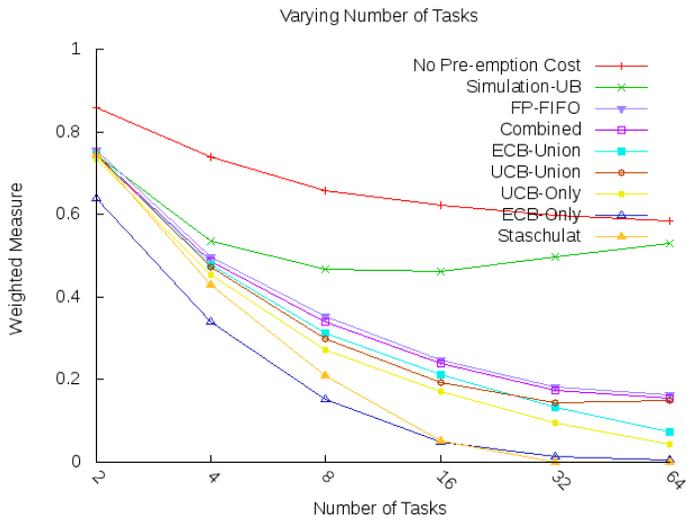
Fig. 25. Weighted schedulability measure; varying number of tasks from  $2 = 2^1$  to  $2^6 = 64$ . (constrained deadline)
