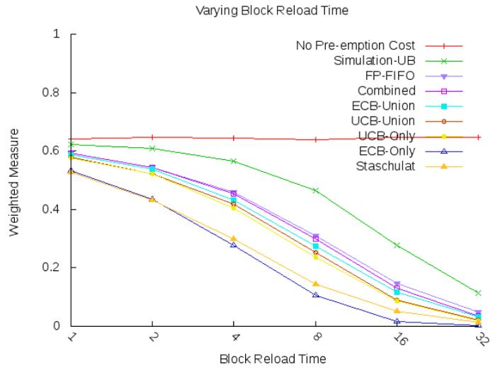
Fig. 27. Weighted schedulability measure; varying block reload time from  $2^0 = 1\mu s$  to  $2^4 = 32\mu s$  (constrained deadline)
