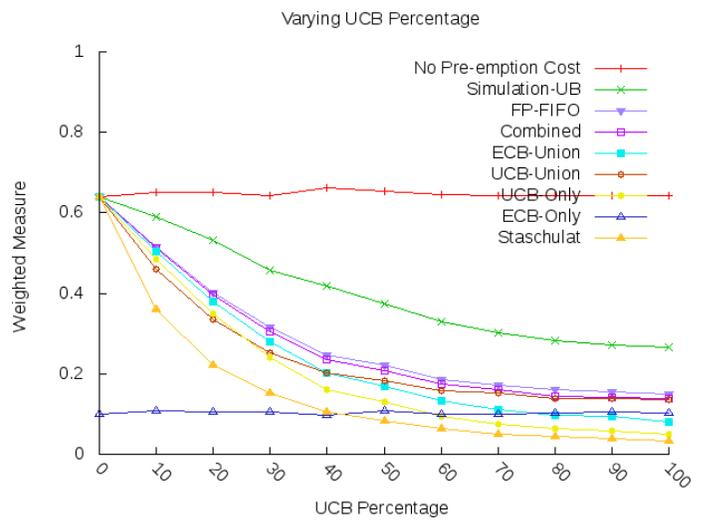
Fig. 24. Weighted schedulability measure; varying reuse factor from 0% to 100%, in steps of 10% (constrained deadline)
