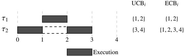
Fig. 1. Taskset  $\{\tau_1, \tau_2\}$  with  $C_1 = 1$ ,  $C_2 = 2$  and block reload time 1. Response time analysis of task  $\tau_2$ : only counting the number of possibly evicted UCBs (4) or possibly evicting ECBs (3) leads to a pre-emption cost of 2, whereas the actual pre-emption cost is 0.
