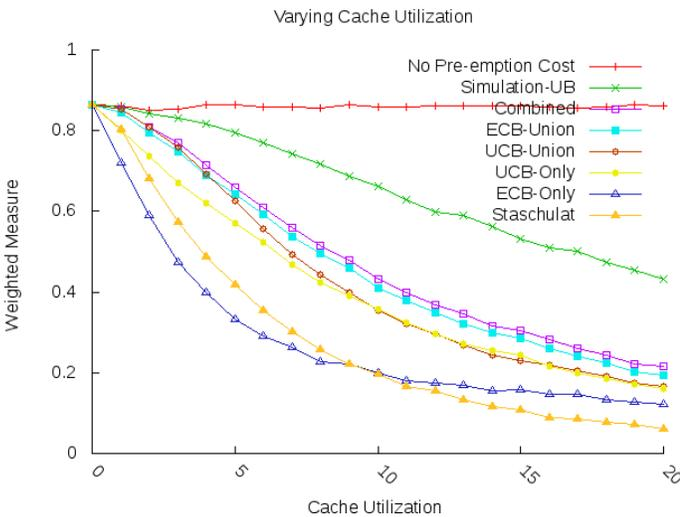
Fig. 7. Weighted schedulability measure; varying cache utilization from 0 to 20, in steps of 2
