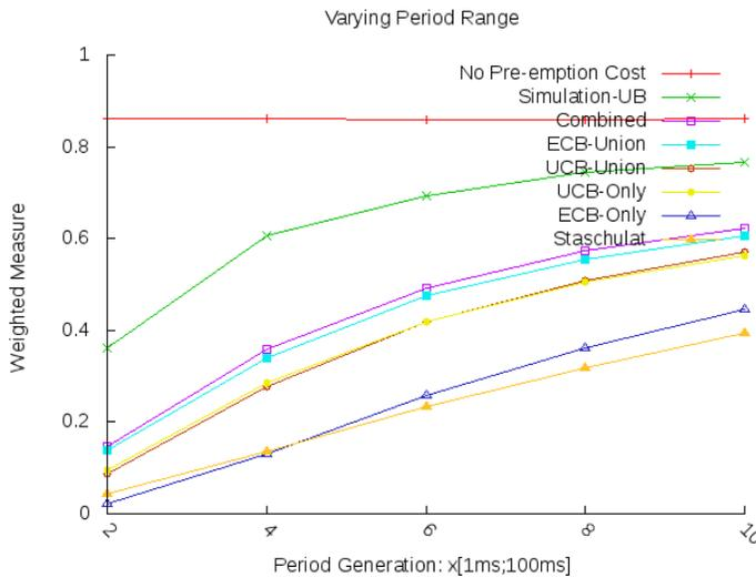
Fig. 13. Weighted schedulability measure; varying the scale of task periods  $w[1, 100]$  from  $w = 2$  to  $w = 10$
