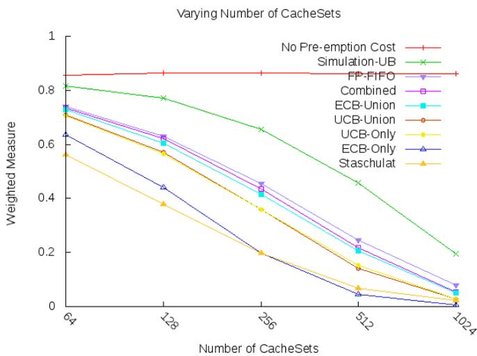
Fig. 18. Weighted schedulability measure; varying number of cache sets from  $2^5 = 64$  to  $2^{10} = 1024$  (with FP-FIFO)
