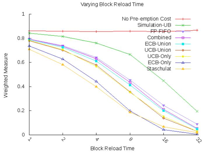
Fig. 19. Weighted schedulability measure; varying block reload time from  $2^0 = 1\mu s$  to  $2^4 = 32\mu s$  (with FP-FIFO)
