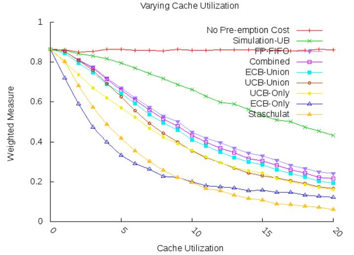
Fig. 15. Weighted schedulability measure; varying cache utilization from 0 to 20, in steps of 2 (with FP-FIFO)
