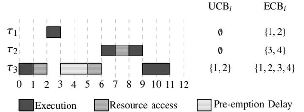
Fig. 5. Tasks  $\tau_2$  and  $\tau_3$  share a common resource  $x$ ,  $\tau_3$  starts to execute, blocks  $\tau_2$ , which is released at time 1, and is pre-empted by  $\tau_1$ . Thus, the finishing time of  $\tau_2$  is delayed not only by the time for which  $\tau_3$  accesses the resource, but also by the additional pre-emption delay, reloading UCBs {1, 2} after the resource access of task  $\tau_3$  is pre-empted by task  $\tau_1$ .
