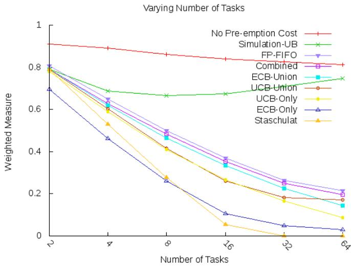
Fig. 17. Weighted schedulability measure; varying number of tasks from  $2 = 2^1$  to  $2^6 = 64$ . (with FP-FIFO)
