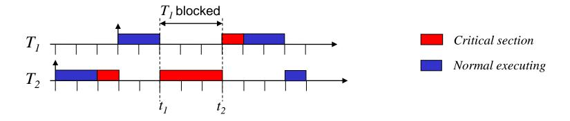
•  $T_2$  is activated first, enters the critical section and locks the semaphore. When  $T_1$  is released, it preempts  $T_2$  since its priority is higher. However, when attempting to enter its critical section at  $t_1$ ,  $T_1$  is blocked on the semaphore, so  $T_2$  resumes – although its priority is lower. In  $[t_1, t_2]$  a priority inversion occurs.
