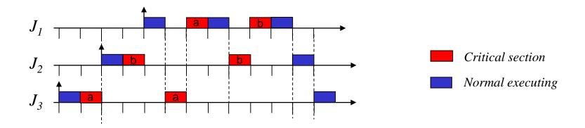
• In the worst case, if  $J_1$  accesses m distinct semaphores that have been locked by m lower-priority jobs, then  $J_1$  will be blocked for the duration of m critical sections.
