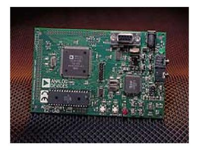
The ADSP-2181-Kit Lite provides an evaluation suite of the VisualDSP++ development environment with the C-compiler, assembler, and linker. Exercises:
